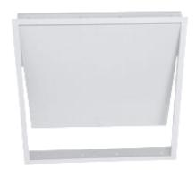
This model of wall and ceiling fire-rated panels is manufactured under the factory inspection service of Intertek Warnock Hersey) and have a label reading: "Listed access frame and insulated fire door assembly 2 hour fire rating. Horizontal Installation Only."
